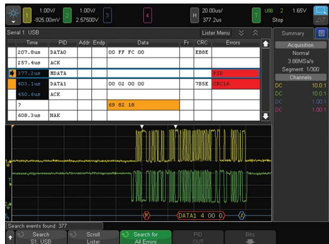
Figure 20: USB 2.0 trigger, decode and “lister” display.
