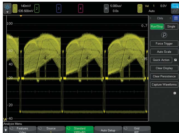
Figure 26: Triggering on 1080p HDTV signal analysis.
